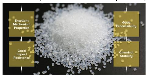
**Available Film Grade:** SM33 = rv.3.23 | SM36 = rv.3.60 **Casting. Biaxial Stretching. Multi-layer**
